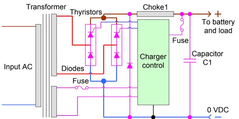
The output of the thyristor controlled bridge rectifier is fed into a critical inductance choke filter to minimise the ripple on the battery and the interference sent back into the AC supply. The output goes to the battery.
