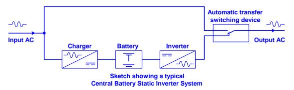
The above sketch shows a typical Static Inverter Central Battery System operating in changeover mode.
